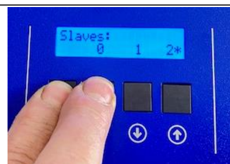
2. Press the two left buttons „ON/OFF“ and „M“ simultaneously
